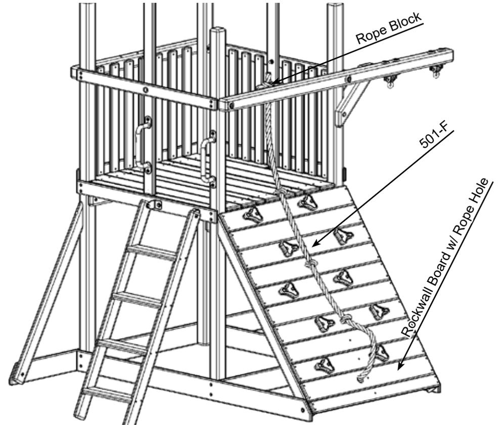
SLIP THE 501-F THROUGH THE ROPE BLOCK AND TIE A KNOT SECURING IT. TIE A COUPLE KNOTS AS YOU WORK YOUR WAY DOWN THE ROCKWALL. SLIP THE 501-F THROUGH THE ROCKWALL BOARD W/ ROPE HOLE AND TIE A KNOT OR 2 SECURING IT.
