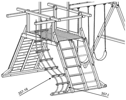
SLIDE ONE END OF ROPE THROUGH THE UPPER ROPE ARM AND TIE A GOOD KNOT. THEN TAKE A 357-16 AND SLIDE IT UP ABOUT A 1 TO 1 1/2 FT BELOW THE ROPE ARM AND TIE KNOT HOLDING IT. REPEAT FOR ALL 357-16'S AND TIE A KNOT ON THE ROPE RUNNER.
