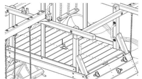
FIND THE CENTER OF THE DECK AND MARK THE HOLES TO BE DRILLED
