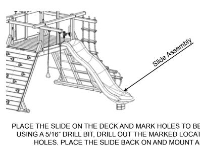
PLACE THE SLIDE ON THE DECK AND MARK HOLES TO BE DRILLED. THEN USING A 5/16" DRILL BIT, DRILL OUT THE MARKED LOCATIONS FOR THE HOLES. PLACE THE SLIDE BACK ON AND MOUNT AS SHOWN
