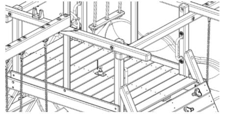
USING A 9/16" BIT DRILL THROUGH THE DECK ON THE MARKED HOLES
