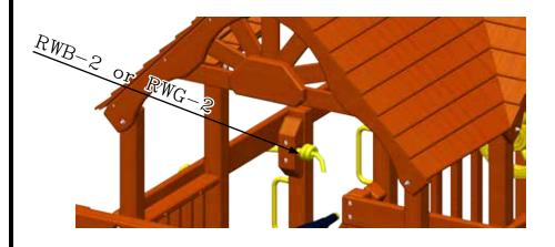
String the rope through Universal Rope Block on the Fort tie a knot securing it in the rope block. Now tie a knot every 2 to 3 ft. until you can string through the RW Board w/ Rope Hole. Tie a knot securing it to the the board.
